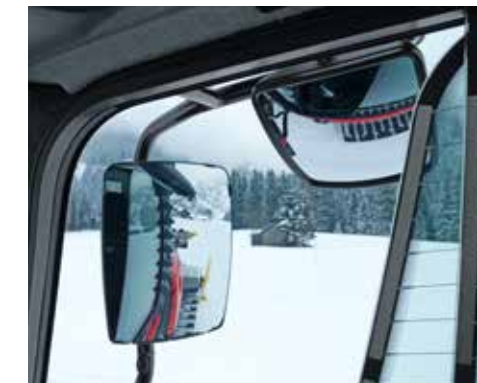
Horizontal mount mirror provides direct view of the tracks.
