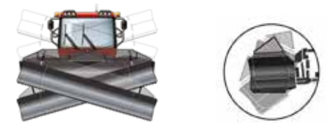
The maximum flexibility of the All-Way-Blade facilitates precise shaping of particular designs.
